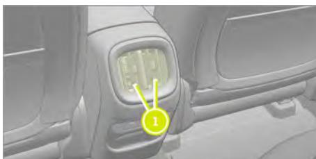
1. **Adjusting the rear air outlet:** move the slider 1 up, down, left and right. Turn the slider 1 down to the maximum position to close the air outlet.
