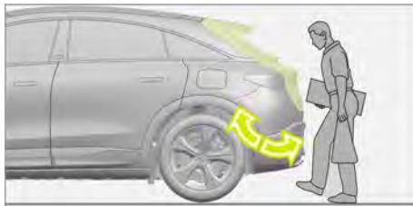
When the vehicle detects the keyfob or smart APP Bluetooth key, you can open, close, or stop the liftgate by kicking below the rear bumper.
