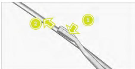
3. Hold the wiper arm with one hand, press the clip inward along the direction of the arrow 1, and pull the blade out along the direction of the arrow 2 with the other hand.
