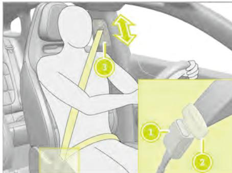
1. Always insert a seat belt tongue 2 into the buckle 1 of the corresponding seat.
