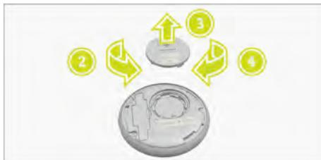
2. Insert a suitable tool into the groove of the battery compartment cover and turn in the direction of the arrow ② to the Open position, then remove the cover ③.
