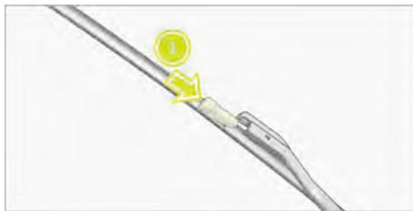
1. Align a new wiper blade with the wiper arm along the direction of the arrow 1 and slide the clip into the locked position.
