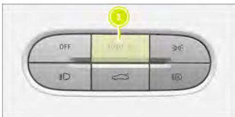
Press the button 1 on the instrument panel combination switch on the driver side to turn on the automatic headlamps.
