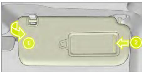
Pull it out from the retainer in the direction of the arrow 1 and swing it toward the door.
