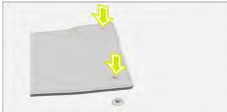
When installing the floor mats, place the floor mats in the correct position, align the floor mat eyelets with the floor mat retaining clips, and then press to lock.
