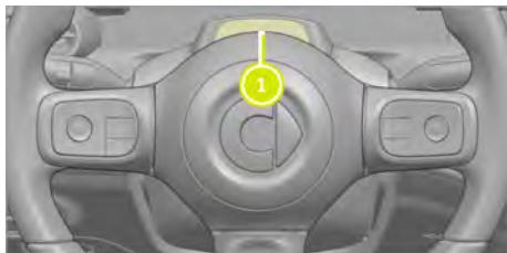
The Driver Monitoring System camera ① is located on the steering column at the rear of the steering wheel.
