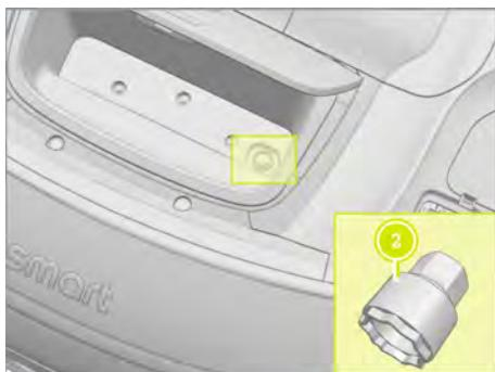
3. Remove the tool kit, flip open the foam base at the button of the front compartment, and then take out the anti-theft wheel bolt adapter ② at the location shown in the figure.
