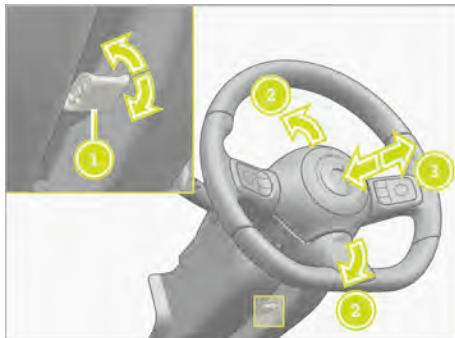
1. Fold down the lever ① to unlock the steering column.
