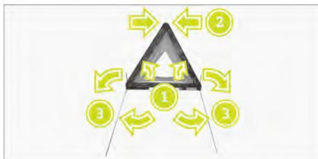
1. Fold the side reflector 1 up to form a triangle and snap on its top with the upper clip 2.
