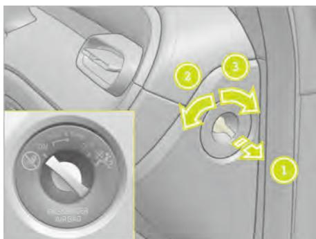
**To enable the passenger airbag:** pull the switch **1** in the direction of the arrow and rotate the switch counter-clockwise **2** to enable the passenger airbag.
