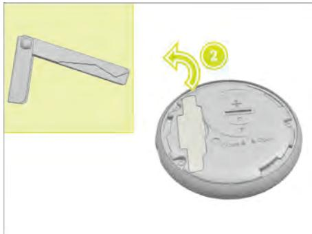
2. Open the mechanical key cover in the direction of the arrow 2 and take out the mechanical key.
