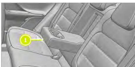
Pull the rope loop 1 outward to expand the second row seat armrest.
