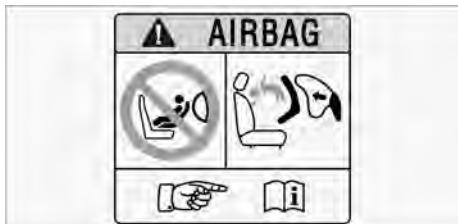
The passenger airbag label is located on the front passenger sun visor.
