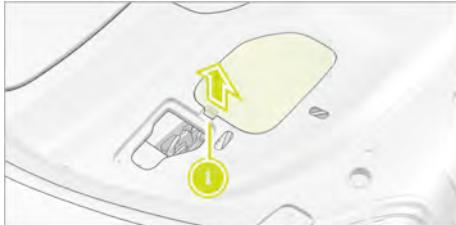
2. Push away the clip 1 and remove the cover along the direction of the arrow.
