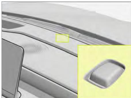
The light sensor is located in the centre of the instrument panel, and the automatic wipers/automatic headlamp/automatic air conditioning control the corresponding functions through this sensor.
