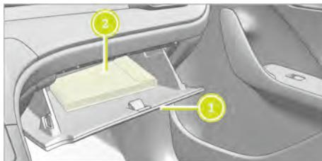
1. **To remove:** open the glove box 1 and take out the safety vest bag 2.
