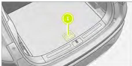
1. To **open**: pull the handle (1) upward and lift the boot floor cover upward.
