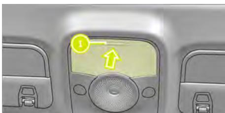
Press 1 in the direction of the arrow to open the glasses box in the centre of the headliner.
