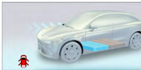
When charging/discharging the vehicle, if any of the doors, the bonnet, the liftgate or the charging port cover is opened, the indicator on the driver information display illuminates to remind the driver of the status of the corresponding door.
