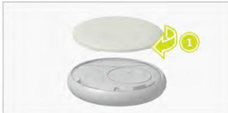
1. Turn the keyfob lower cover in the direction of the arrow 1 and remove it.
