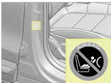
The label is visible on the passenger side B pillar when the front passenger door is opened.
